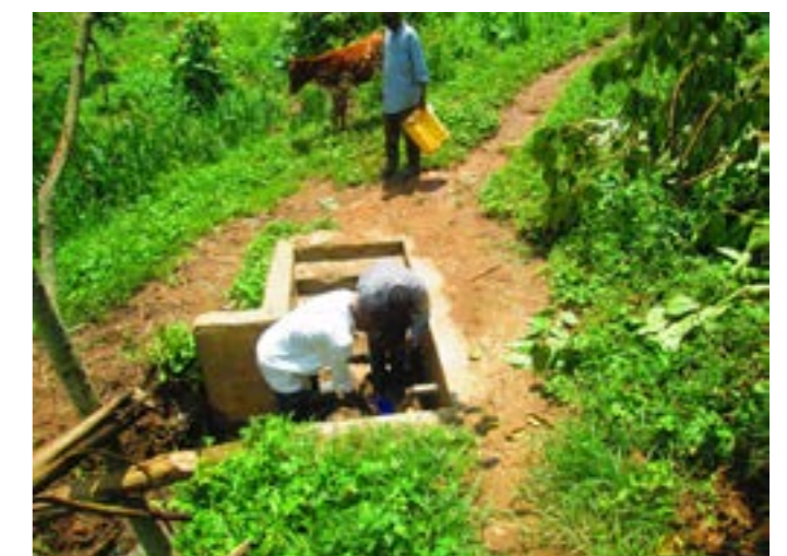
Alex and volunteer taking flow measurements of lower source
